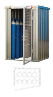
Size Hiltra Gas cylinder depot model GDS-18 Article number 210100260 Dimensions external 1420 x 1030 x 2225 mm **WxDxH** Dimensions internal BxDxH 1300 x 850 x 2080 mm Storage capacity 18x 50 ltr standard cylinder Weight ca.195 kg Compartments Equipment Bottles can be secured in bulk (1 chain over the entire width)
